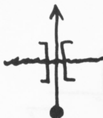
BROKEN BRIDGE OR CULVERT
